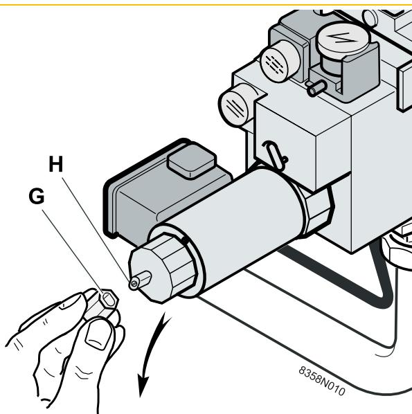
In the factory, the progressivity is set to minimum (low start-up pressure).
