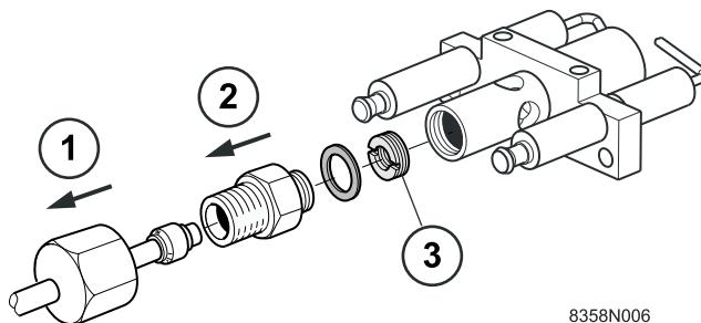
① Remove the gas supply pipe from the ignition burner (13 mm spanner).
