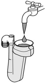
The condensate discharge system, pipework and fittings must be made of plastic. No other materials may be used. The discharge duct must have a minimum gradient of 5 – 20 mm/m throughout its length. Condensate discharge via the gutter is not allowed given the risk of frost and the possible damage to materials
