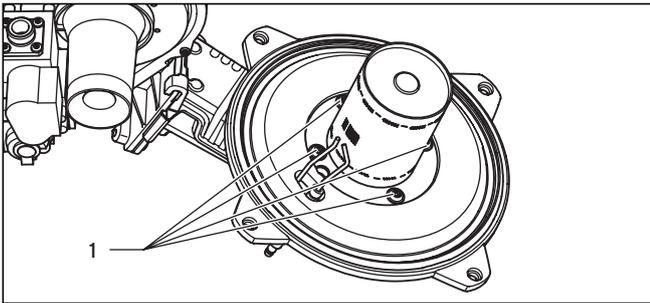
Fig. 9.1 Replacing burner
