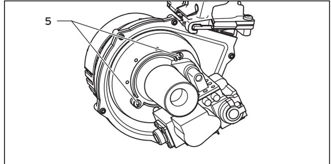
Fig. 9.3 Gas fitting/fan screwed joint
