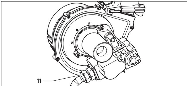
Fig. 7.8 Testing the gas supply for soundness
