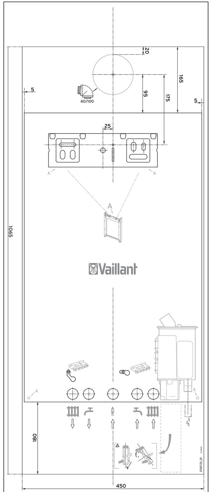
Fig. 4.2 Assembly template
