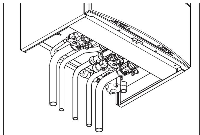
Fig. 5.3 Double check valve detached while heating
