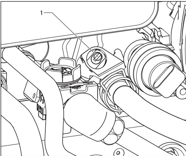
Fig. 5.11 Adjusting the by-pass valve (in combination boilers)
