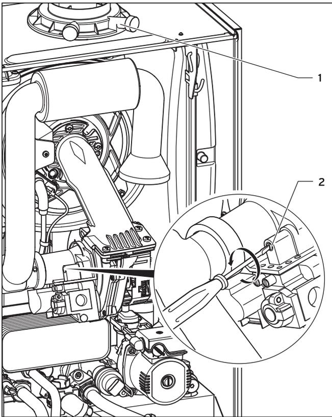
**Fig. 9.7 Carrying out measurement of CO<sub>2</sub> levels, preparing for air-ratio adjustment**
