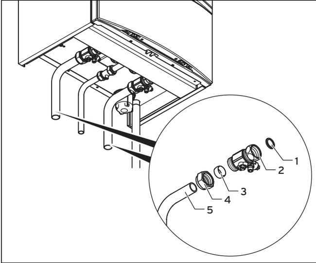
**Fig. 4.11 Heating-side flow and return connection for ecoTEC plus system boiler**
