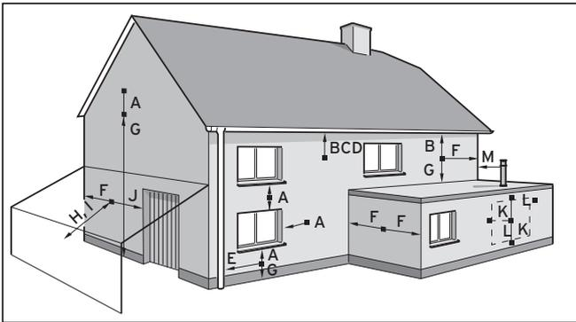
Fig. 3.8 Flue termination
