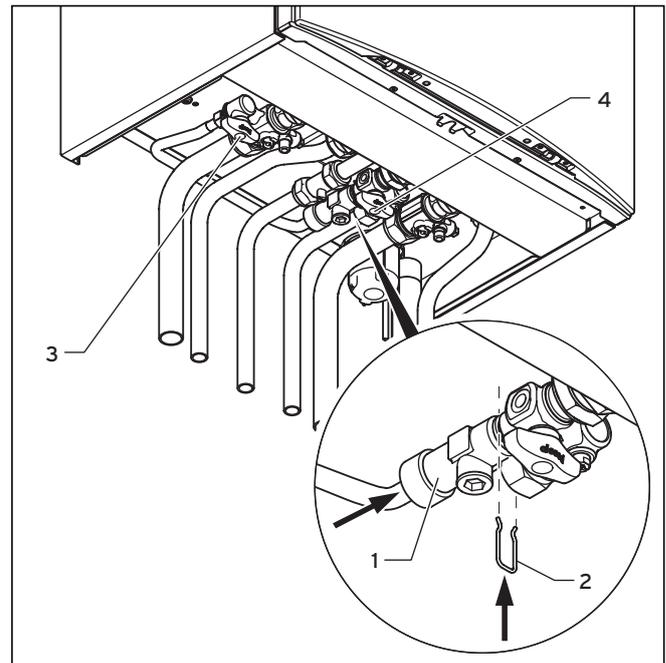
Fig. 5.2 Filling device ecoTEC plus combination boiler
