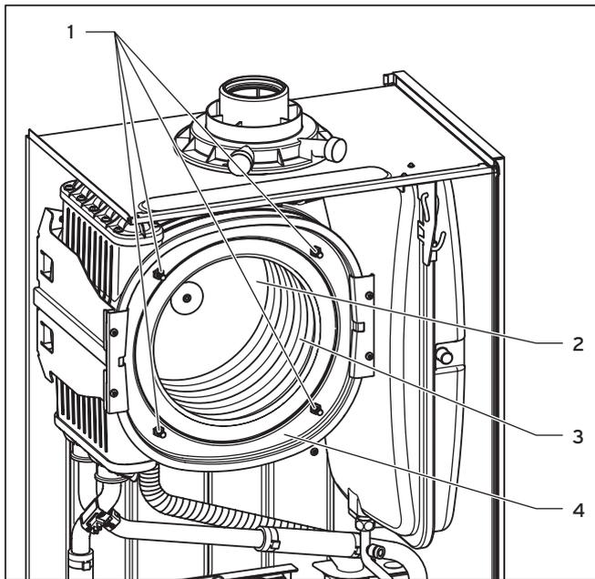
Fig. 7.3 Cleaning the integral condensation heat exchanger
