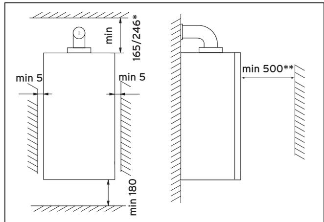
Fig. 4.1 Distances during installation (dimensions in mm)
