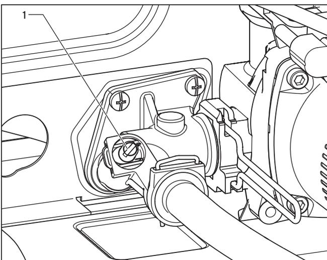
Fig. 5.12 Adjusting the by-pass valve (in system boilers)
