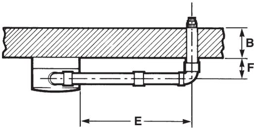
$L = B + E + F + 230 \text{ mm} + (90^\circ \text{ bend} = 1.3 \text{ metre})$
