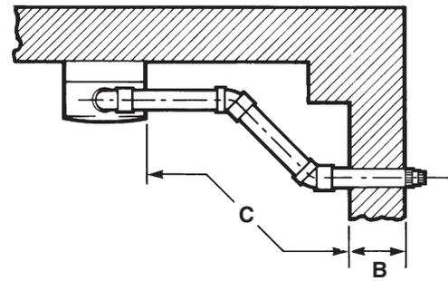
$L = B + C + 230 \text{ mm} + (2 \times 45^\circ \text{ bends} = 1.8 \text{ metre})$
