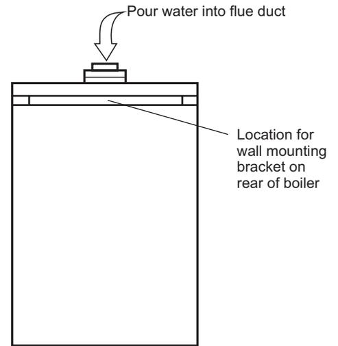
Fig. 4.3 - rear of boiler
