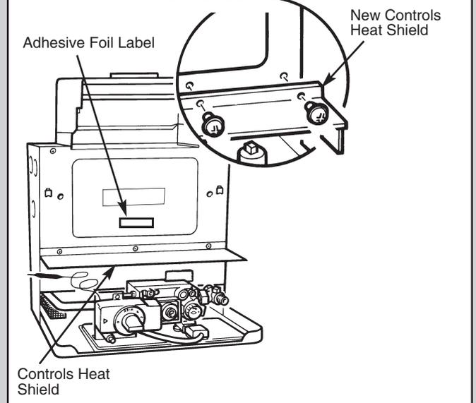
**NOTE: It is important at this stage to fit the controls heat shield supplied with the fire unit to the boiler front panel.**
