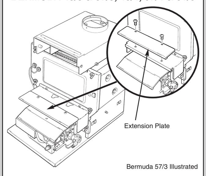
If a radiant firefront has been installed previously it will be necessary to unscrew and remove the extension plate from the boiler controls heat shield. Once removed this item can be discarded.
