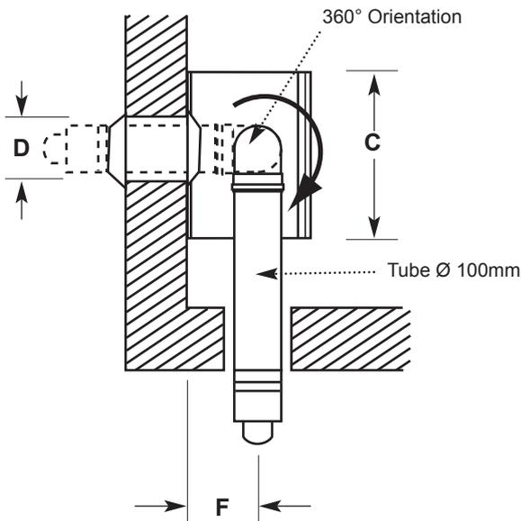
**NOTE:** There must be no part of the air duct (white tube) visible outside the property after installation. The flue seal should fit neatly and effect a good seal.
