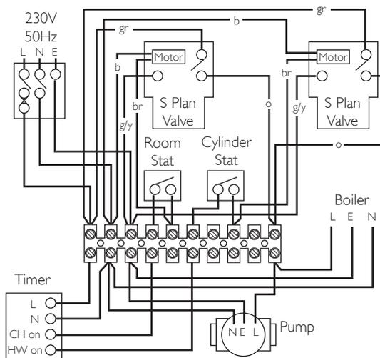
**S Plan, Room Thermostat System, CH Interlocked By Room Thermostat**
