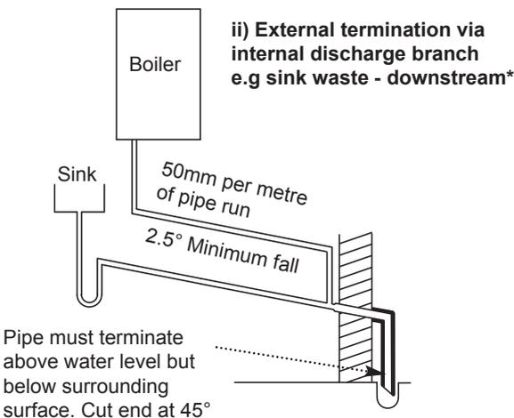
\*It is NOT RECOMMENDED to connect upstream of the sink or other waste water receptacle !
