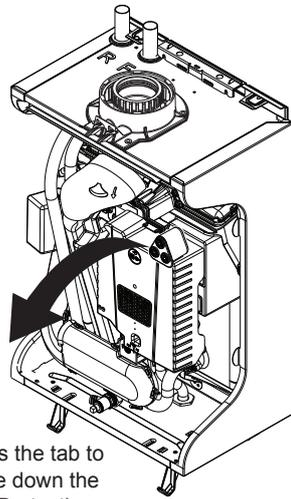
Press the tab to hinge down the Fan Protective Cover
