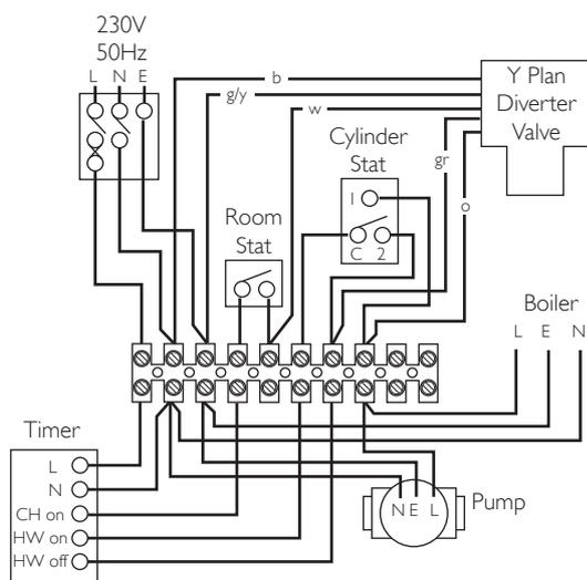
**Y Plan, Room Thermostat System, CH Interlocked By Room Thermostat**
