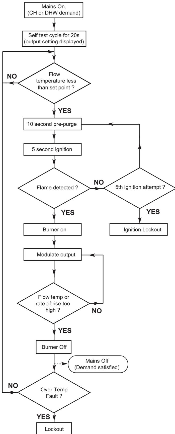
1. **Switched Live On:** When the boiler switched live turns on the boiler, a 20 second check cycle takes place. If the flow temperature is less than the boiler set-point temperature the ignition cycle will start. Pre-purge, Ignition and Burner on.
