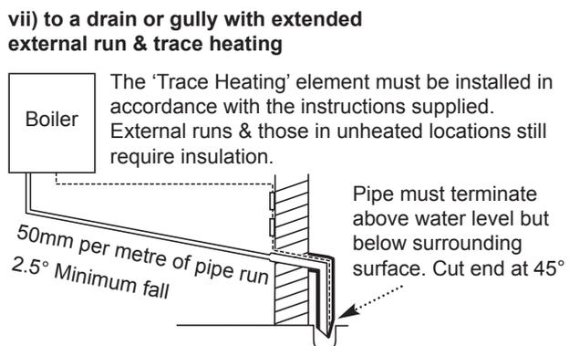
9. If the boiler is fitted in an unheated location the entire condensate discharge pipe should be treated as an external run and sized and insulated accordingly.
