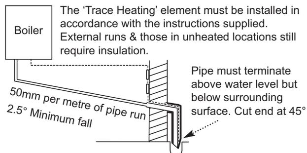
The 'Trace Heating' element must be installed in accordance with the instructions supplied. External runs & those in unheated locations still require insulation.
