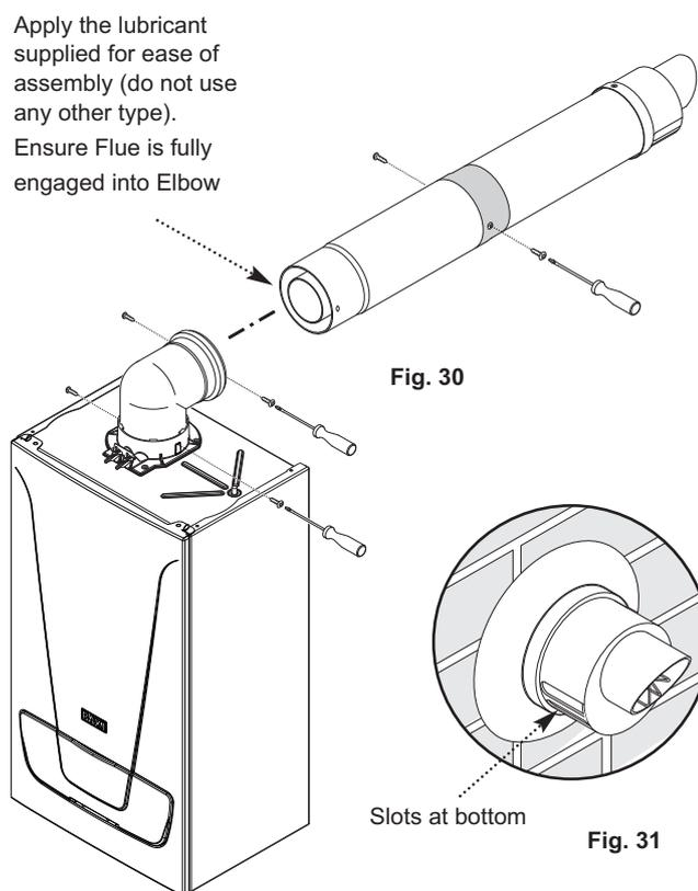
10. Remove the flue elbow and insert the flue through the hole in the wall. Fit the flue trims if required, and refit the elbow to the boiler adaptor, ensuring that it is pushed fully in. Secure the elbow with the screws supplied in the boiler fitting kit (Fig. 29).
