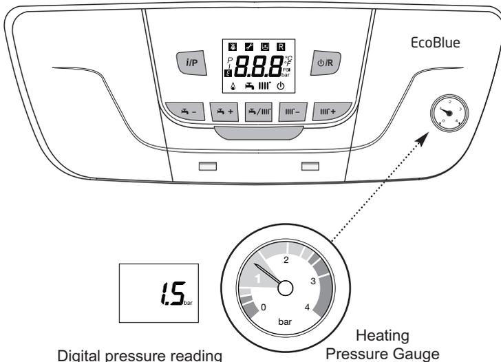
Digital pressure reading which can be accessed by via the **iP** button and scrolling to setting '5'. Note there may be a slight difference between the digital & gauge reading depending on boiler operating mode.
