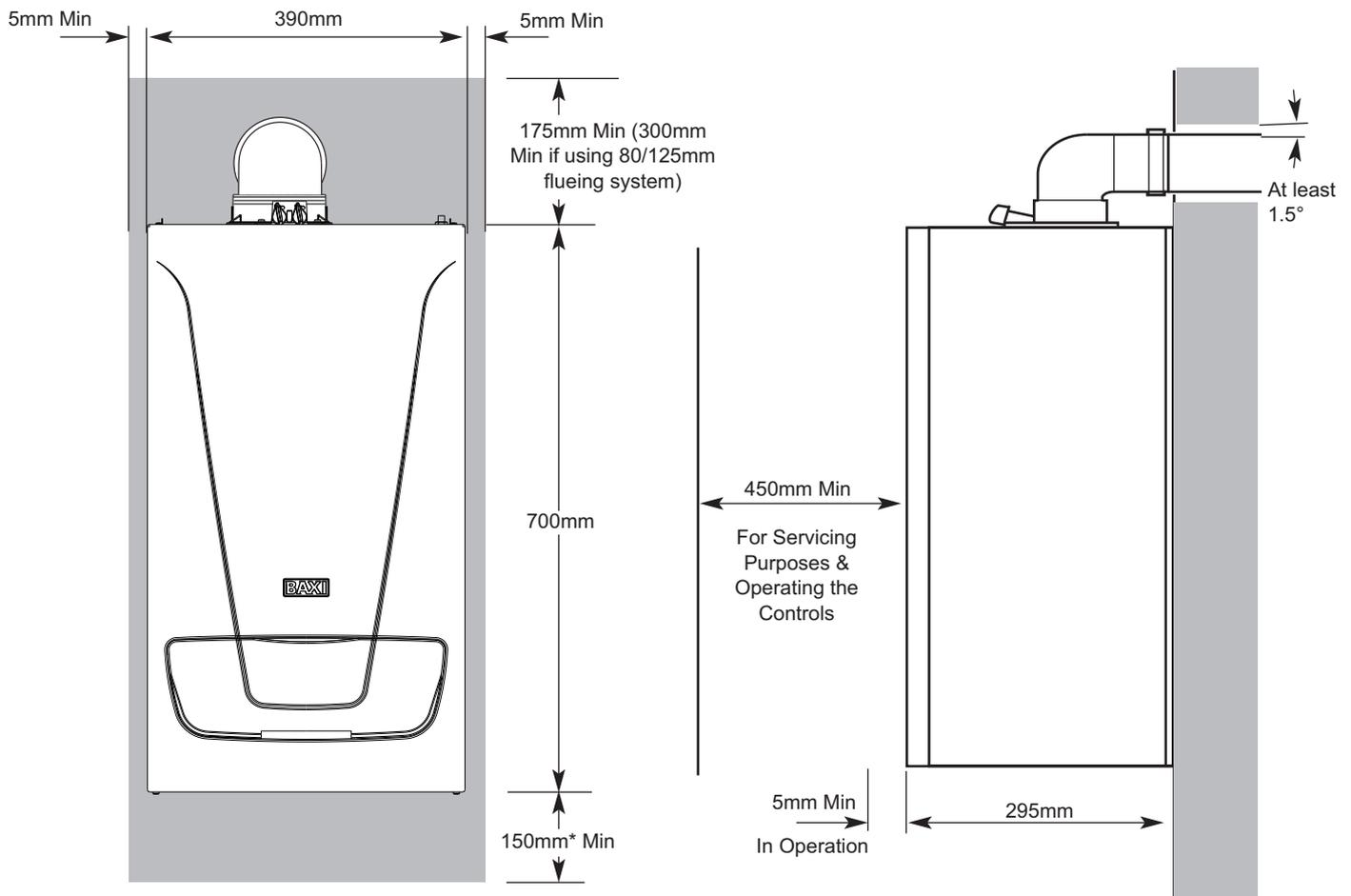
\*This is MINIMUM recommended dimension. Greater clearance will aid installation and maintenance.
