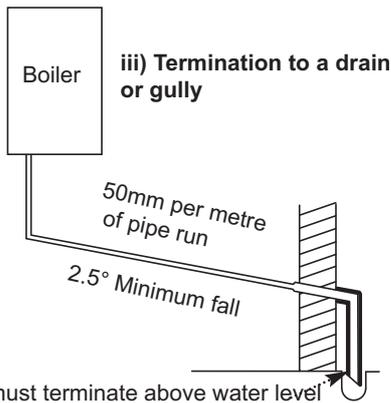
Pipe must terminate above water level but below surrounding surface. Cut end at 45°
