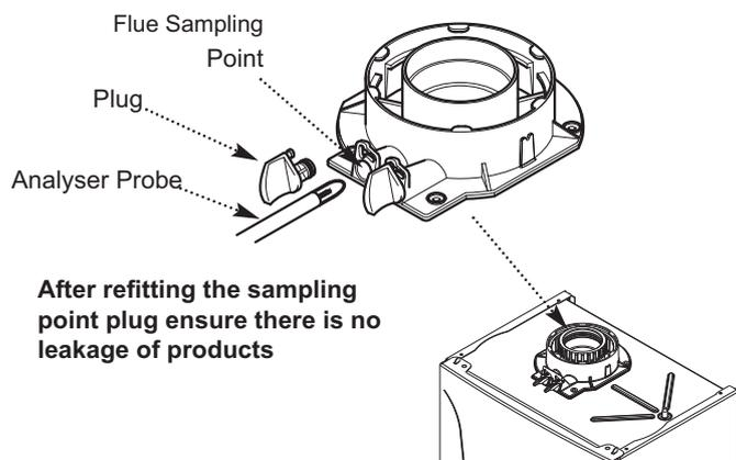
After refitting the sampling point plug ensure there is no leakage of products
