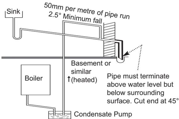
Pipe must terminate above water level but below surrounding surface. Cut end at 45°
