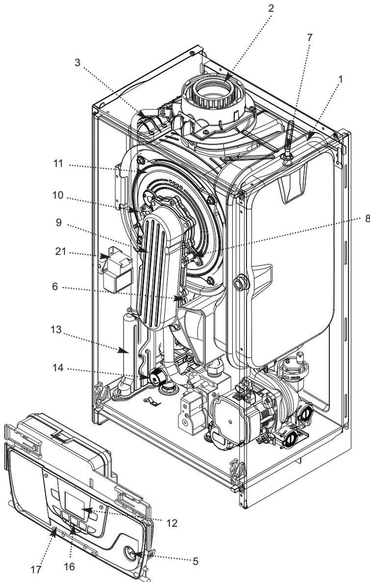
1. Expansion Vessel (Note: This component is at the left on 32 model)
