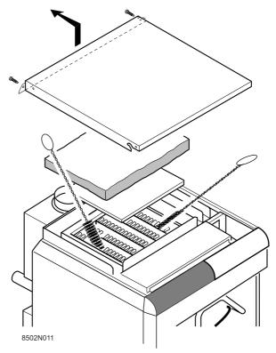
The extent of clogging on the heating body must be checked once a year.
