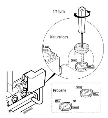
If necessary, the start-up pressure can be set on the **right valve (1st stage)** using a flat screwdriver.
