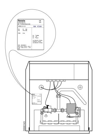
The rating plate affixed to the front panel during assembly provides the exact identification of the boiler and indicates its principal characteristics.
