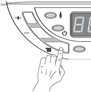
Press on key 32
