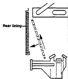
**To replace combustion chamber linings**
