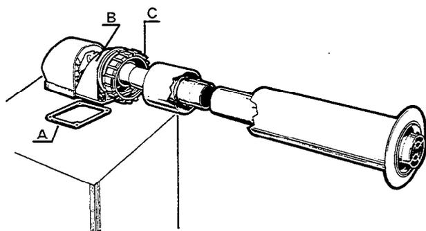
**Fitting the flue 600 mm long or less**
