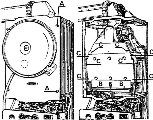
**Remove combustion chamber front panel**
