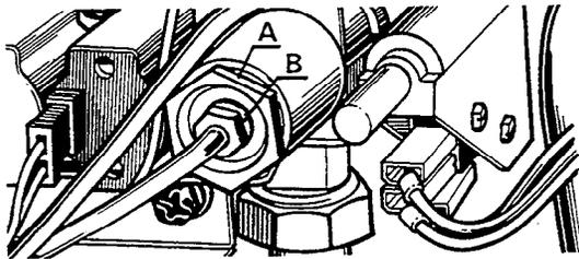
**To replace thermoelectric valve**
