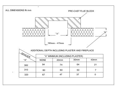
Fireplace opening must be 552 mm - 578 mm high by 380 mm - 435 mm wide (or up to 458 mm if the cable fixing system is used).
