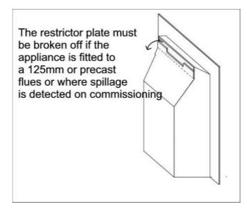
A pre-cast flue conforming to the requirements of BS 1289 part 1 & 2 A suitable fire resisting fire surround will be required, spaced out to the correct thickness, between the face of the flue blocks and the rear of the appliance frame. IMPORTANT: - the flue restrictor plate must not be fitted when the appliance is installed in this type of flue.
