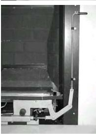
Connect the link lever to the stud at the end of the slide control lever and replace the nyloc nut. IMPORTANT TURN THE NUT UNTIL IT JUST TIGHTENS AND THEN TURN IT BACK A HALF TURN.
