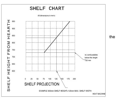
side forward projection is increased by 12.5 mm add 50 mm to inside width of surround.
