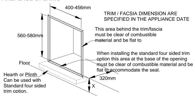
The front face and the base of the fire opening must be flat to ensure that a good seal is formed between the rear and base of the appliance and the chimney to avoid any reduction of natural draught.
