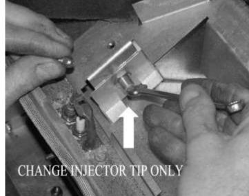
Retighten the two screws and ensure the burner bar is central and flat to the burner carrier.
