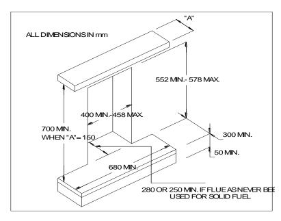
Fireplace opening must be 552 mm - 578 mm high by 400 mm - 435 mm wide (or up to 458 mm if the cable fixing system is used).
