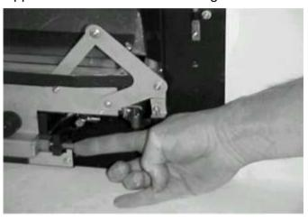
Ensure the spindle is pushed back inside the control valve as far as possible. Ensure the bell crank mechanism is swung up to give easy access to the gas connection point as shown.
