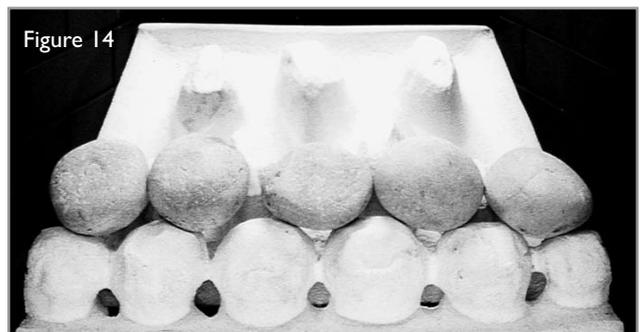
3. Take five more ceramic pebbles and position as shown to form the 'second row' of the fuel effect as shown in figure 15. The pebbles may be rotated as desired to fit into the gaps between the supports in order to create a random, realistic effect. Again, remember not to push the pebbles down too far into the valleys between the supports as this can have a detrimental effect to the flame picture.
