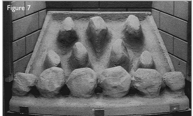
3. Coals. All of the coals are the same. Take five coals and place them as shown in figure 9. Care should be taken to ensure that the coals bridge the gap between the front coal and the four coal supports at the front of the matrix. Care should also be taken not to push the coals right down between the coal supports, as this can detract from the flame picture when the appliance is running.
