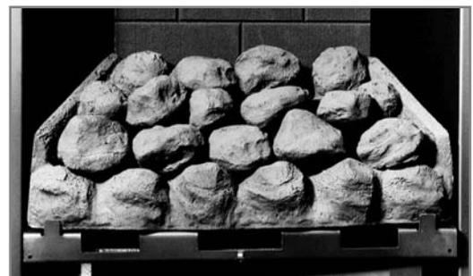
The coals may be rotated slightly within their positions to give a good visual effect. Pay special attention to finally adjust the coals with the fire lit on the HIGH setting in order to ensure that no flames play onto the firebox sides. This will reduce the possibility of heat discolouration.
