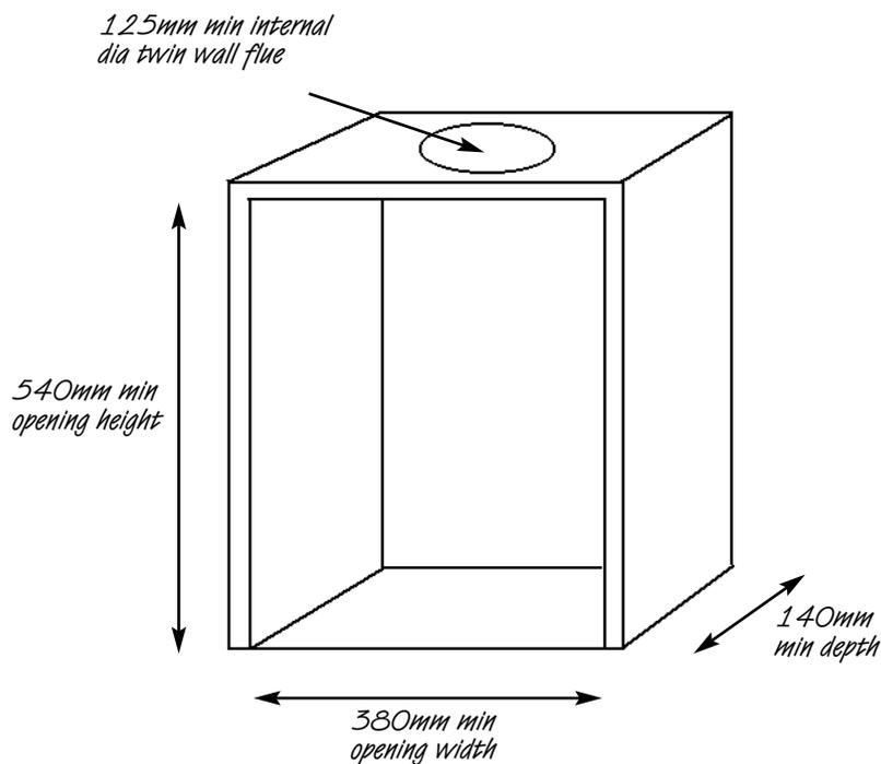
To fit the fire using the cable fixing kit, some minor adaption may be necessary for certain flue boxes. A check should be made to ensure the firebox does not obscure the flue box outlet.
