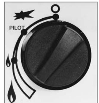
To achieve the HIGH setting, push the control knob in slightly and continue turning anti-clockwise to the high position. The main burner should light after a few seconds. To decrease the setting to LOW, turn the control knob clockwise to the low setting.
