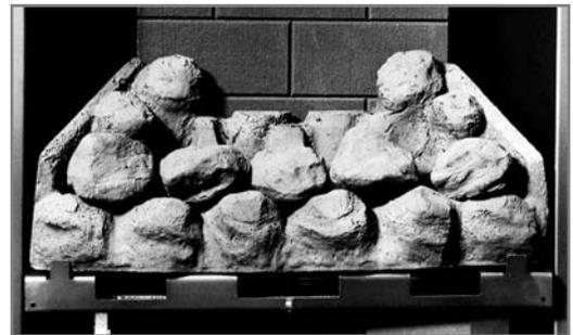
Place the front row of five coals on to the matrix. Ensure the coals are firmly against the side cheeks as shown in the photograph. If necessary, pull the coals forward slightly to ensure their rear edges do not overhang the flame ports. The edges of the coals **MUST NOT** be allowed to enter the flame ports.
