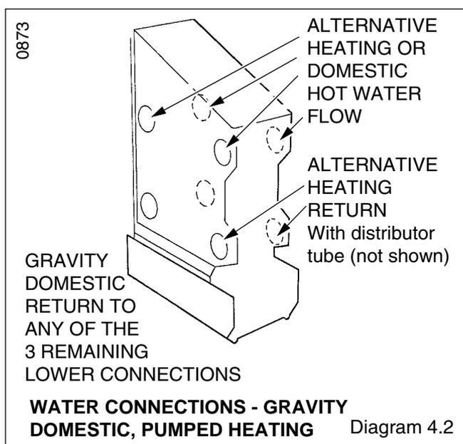
WATER CONNECTIONS - GRAVITY DOMESTIC, PUMPED HEATING Diagram 4.2
