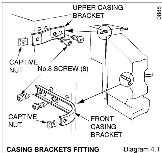
CASING BRACKETS FITTING Diagram 4.1
