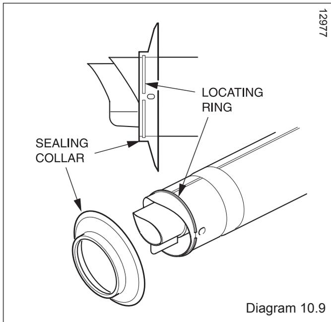
With the flue elbow removed, push the flue assembly into the wall, externally or internally, until the end of the assembly protrudes a short way from the inside face of the wall. This will enable the internal trim ring (if required) to be positioned and allow the flue assembly to be drawn back up to the flue elbow.
