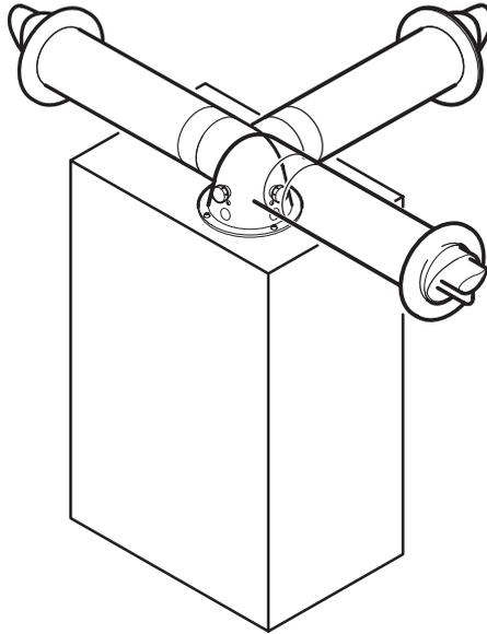
**Top horizontal standard flue (Ø60/100)**
