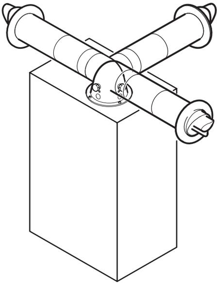
**Top horizontal telescopic flue (Ø60/100)**
