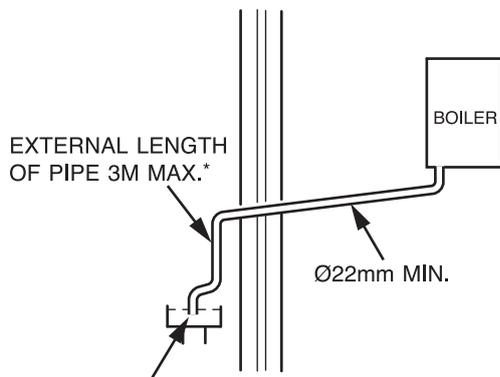
OPEN END OF PIPE DIRECT INTO GULLEY BELOW GROUND BUT ABOVE WATER LEVEL
