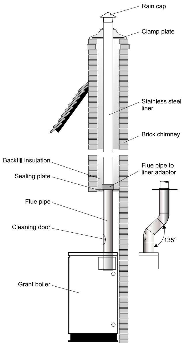
Fig. 10 - Typical conventional flue with brick chimney
