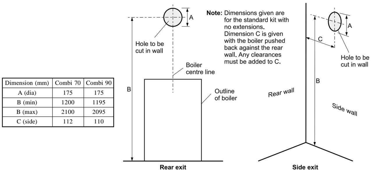
**Fig. 14 - High level balanced flue**
