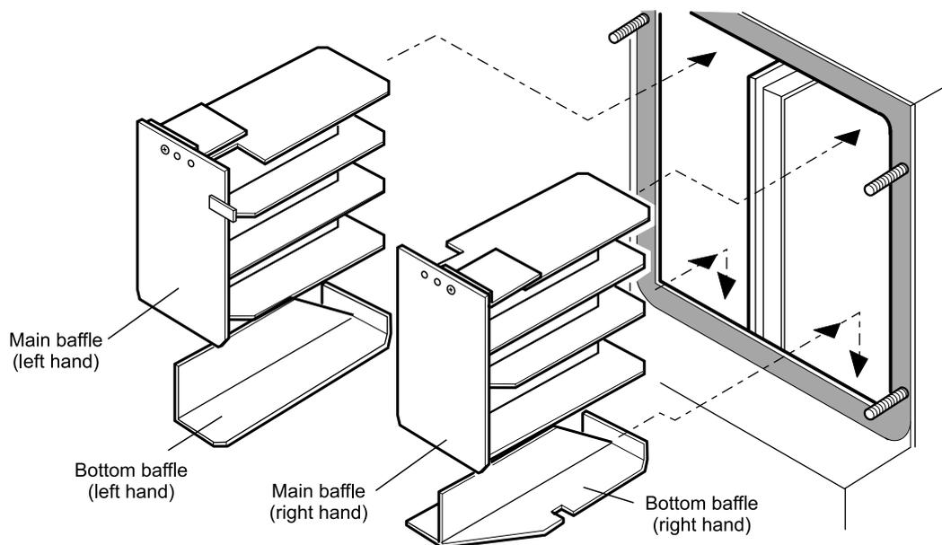
Fig. 34 - Combi 90 baffle positions
