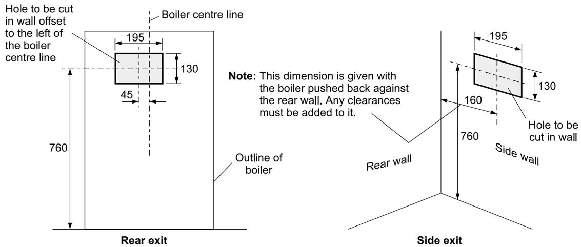
**Fig. 13 - Square low level balanced flue**
