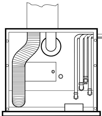
**Fig. 18 - Combi 70 pipework/flue configurations (square flue)**
