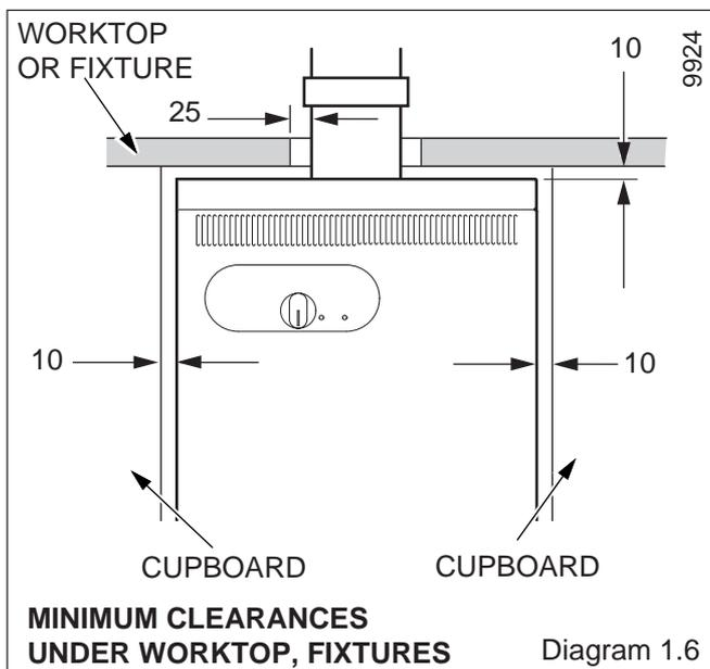
The boiler may be installed in any room, although particular attention is drawn to the requirements of BS7671 with respect to the installation of a boiler in a room containing a bath or shower. Any electrical switch should be so positioned that it cannot be touched by a person using the bath or shower. The electrical provisions of the Building Standards (Scotland) Regulations apply to such installations in Scotland.
