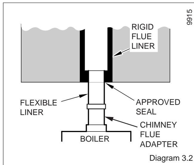
In the case of a salt glazed flue, it is recommended that a short vertical length of flue pipe be connected in such a manner that any condensation from the flue is not retained. Fix and seal it to the boiler flue socket and make good with an approved seal. It is also recommended that a permanent drain be fitted to the boiler.
