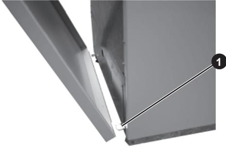
2. Loosen 3 screws on one side of the inner front panel and undo the 3 screws from the other side. The panel will now slide to one side for removal.
