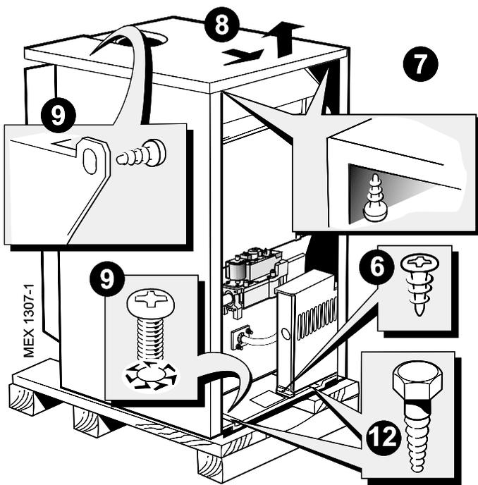
6. Release the screw securing the control box to the baseplate and slide to the left to release the box.
