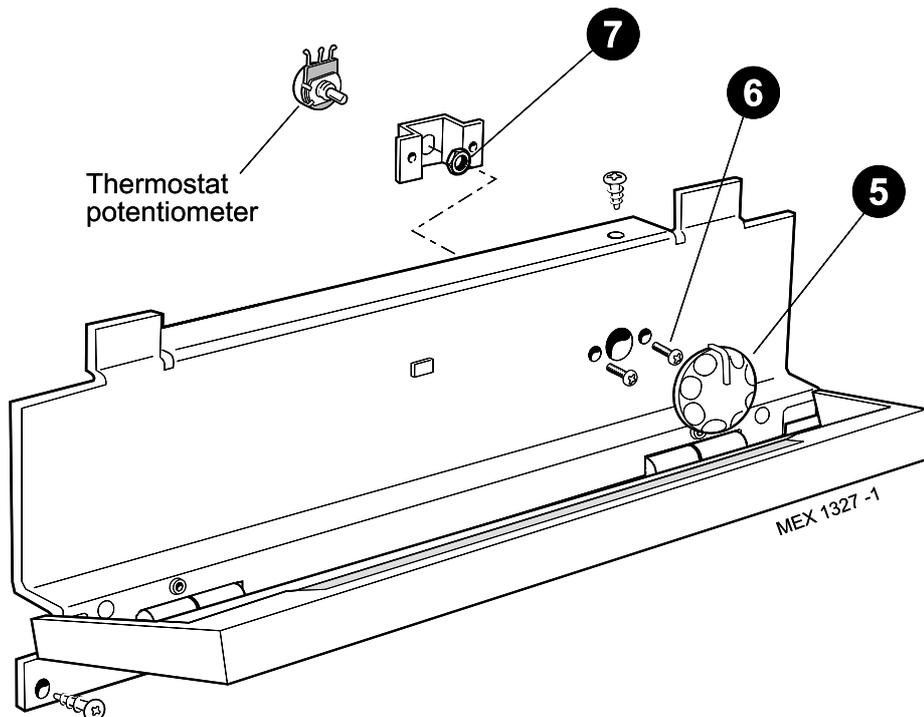
1. Remove the lower front panel and grille assembly. Refer to Frame 47.
