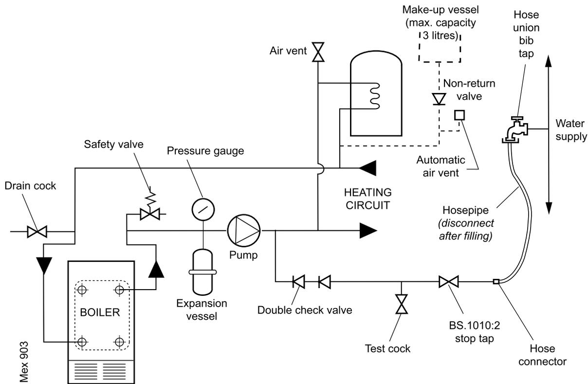
**Note.** The method of filling, refilling, topping up or flushing sealed primary hot water circuits from the mains via a temporary hose connection is only allowed if acceptable to the local water authority.
