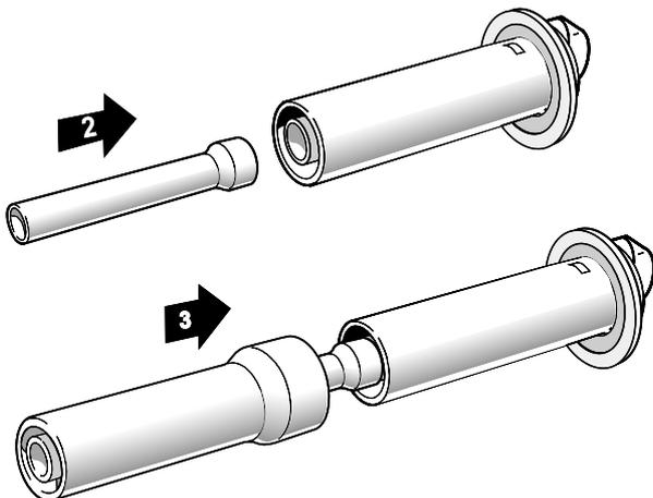
2. Fit the inner flue extension duct onto the inner flue duct.
