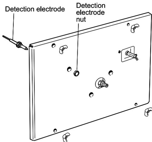
1. Remove the lower front panel/grille assembly. Refer to Frame 47.
