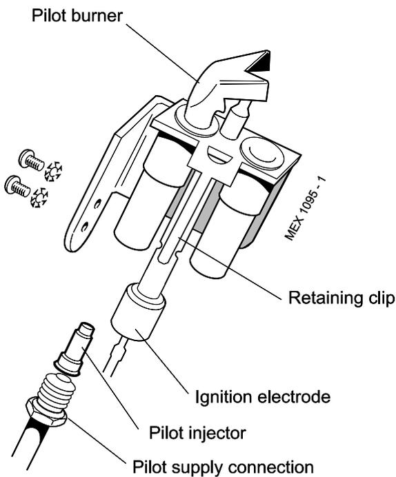
1. Remove the 2 screws and lift off the lower front panel then remove the grille assembly. Refer to Frames 57. Undo the gas cock union. Remove the 4 wing nuts and withdraw the burner and controls assembly, complete, from the boiler.
