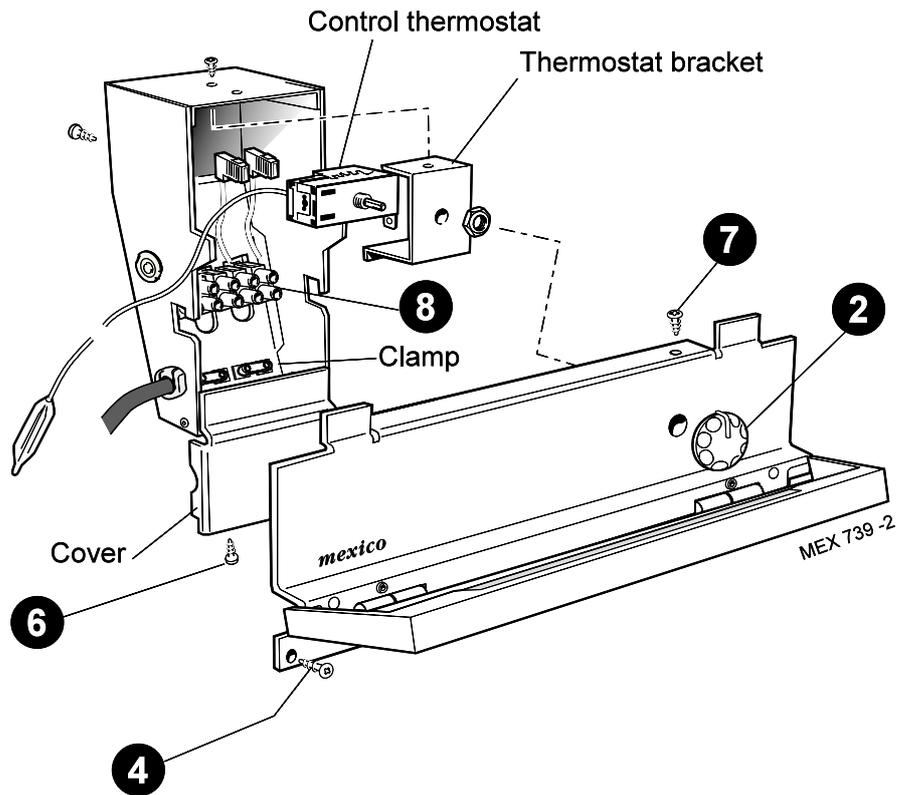
13. Replace the lower front panel and secure with the 2 fixing screws.
