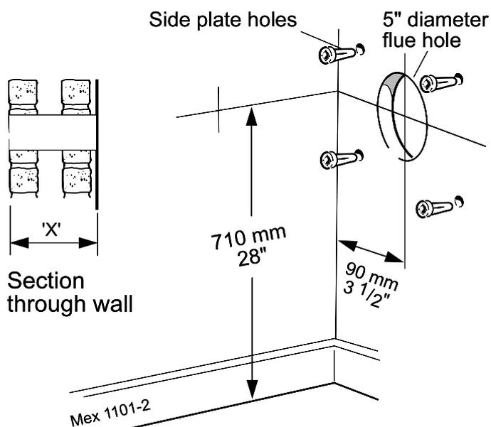
**Note.** If the terminal is to be sited within 25-40mm of a corner or vertical pipe (refer to Table 3) then the hole **MUST** be accurately cut and the rubber weather seal trimmed around the groove provided. The terminal wall plate need not be fitted.
