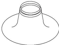
Flue Seal Collar - Tile Roof
