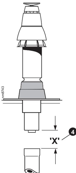
4. If the last extension duct requires cutting, measure 'X', the distance (outer ducts), between the duct and the terminal and add 100 mm to this dimension. This gives the length of the last extension duct.
