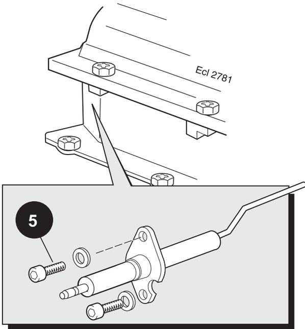
5. Remove the flame detection electrode.
