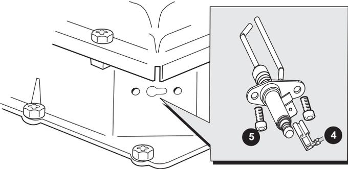
7. Fit the new ignition electrode, using the new gasket supplied. Check dimensions as shown.
