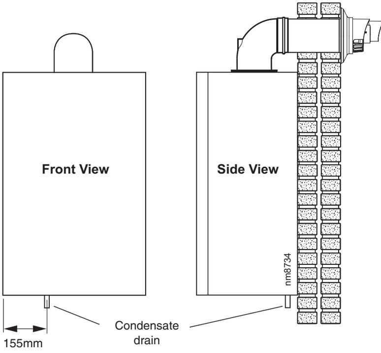
The condensate drain provided on the boiler must be connected to a drainage point, preferably within the building.
