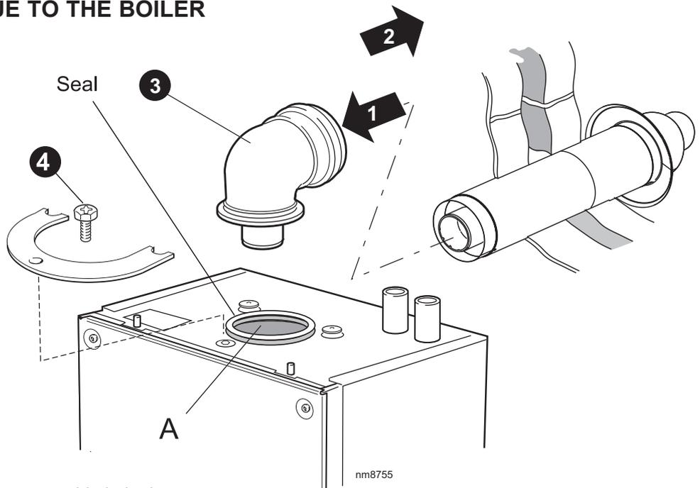
1. Locate the flue into the turret.
