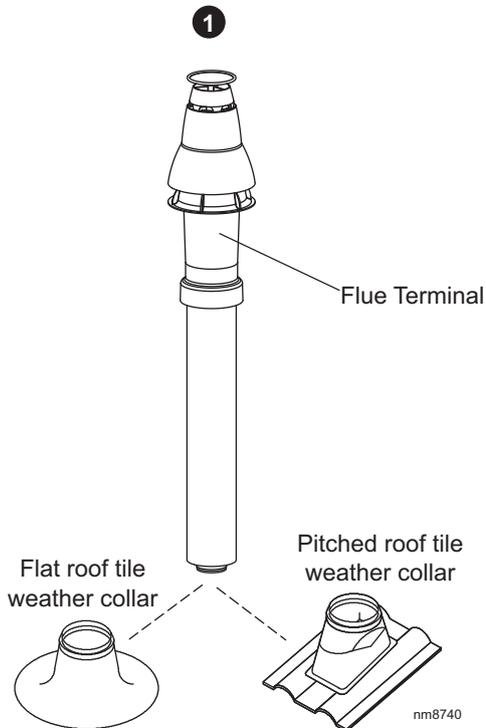
2. Push fit the vertical connector (supplied separately) into the boiler flue connection and retain with the turret clamp and securing screw (supplied with the boiler). **ENSURING THE GASKETS IN THE BOILER FLUE OUTLET ARE CORRECTLY FITTED.**
