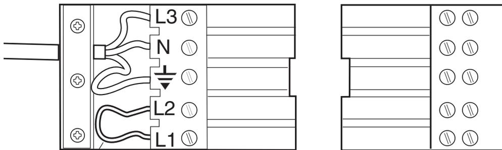
Remove link when connecting external programmer.
