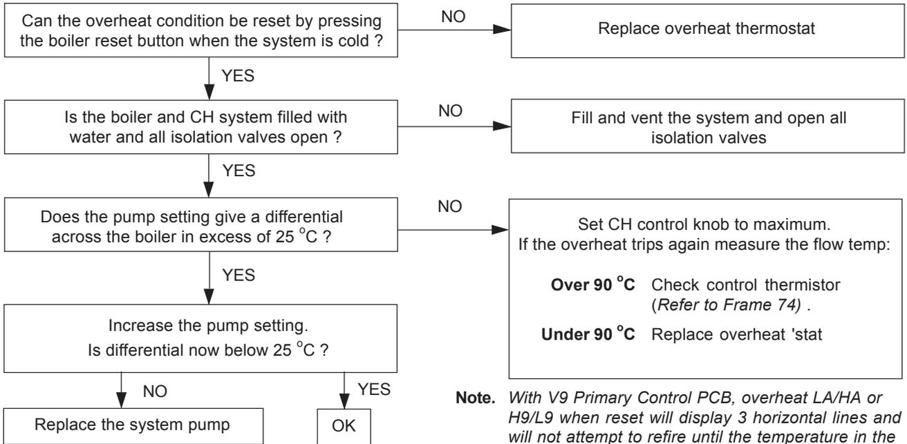
**Note.** With V9 Primary Control PCB, overheat LA/HA or H9/L9 when reset will display 3 horizontal lines and will not attempt to re-fire until the temperature in the heat exchanger drops below 50°C.
