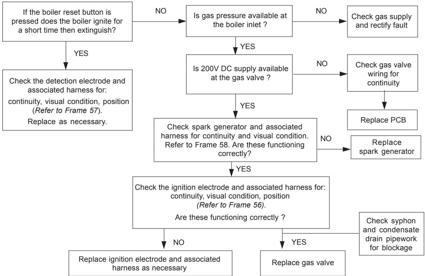
**Note.** Due to the wave form of the rectified voltage the reading will vary, depending on the type of meter used to measure the value (some may measure the possible peak voltage of 339V). In general terms, a reading greater than 150V indicates that the correct voltage is supplied to the gas valve. As an alternative to a multimeter a mains checking device may be used. E.g. an electrical screwdriver or a mains tester.
