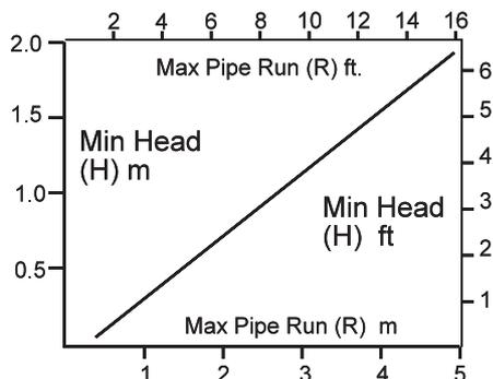
The above graph assumes 8 elbows in the gravity circuit. For each elbow in excess of 8, (R) must be reduced by 300 mm (12 in.) or (H) increased by 100 mm (4 in.)
