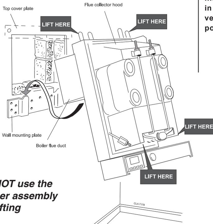
**Do NOT use the burner assembly for lifting**
