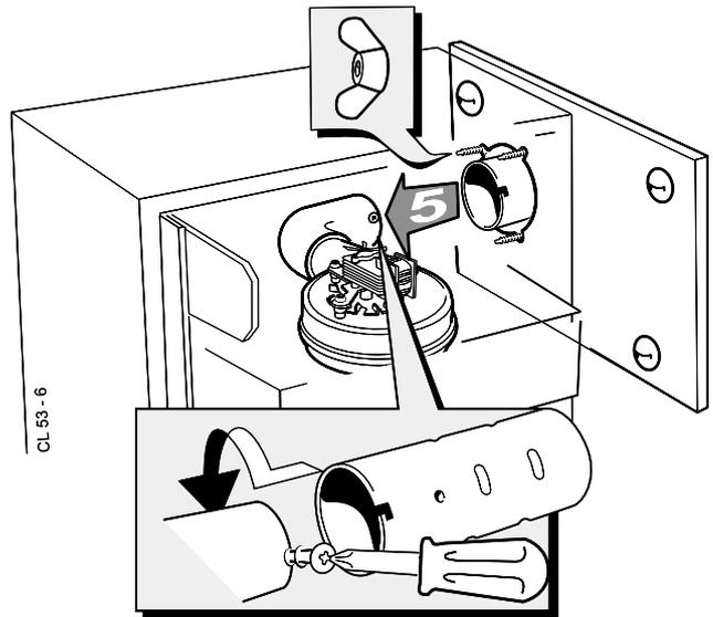
**Note.** The sealing ring studs will locate in the back panel one way only. This will ensure that the terminal grille is correctly aligned.
