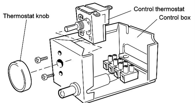
6. Remove the 2 screws securing the thermostat.
