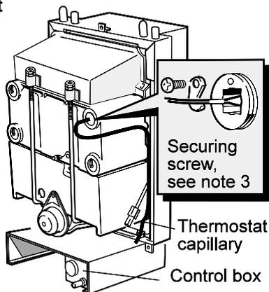
5. Remove the control box fixing screw and pull the box forward and downward to disengage.
