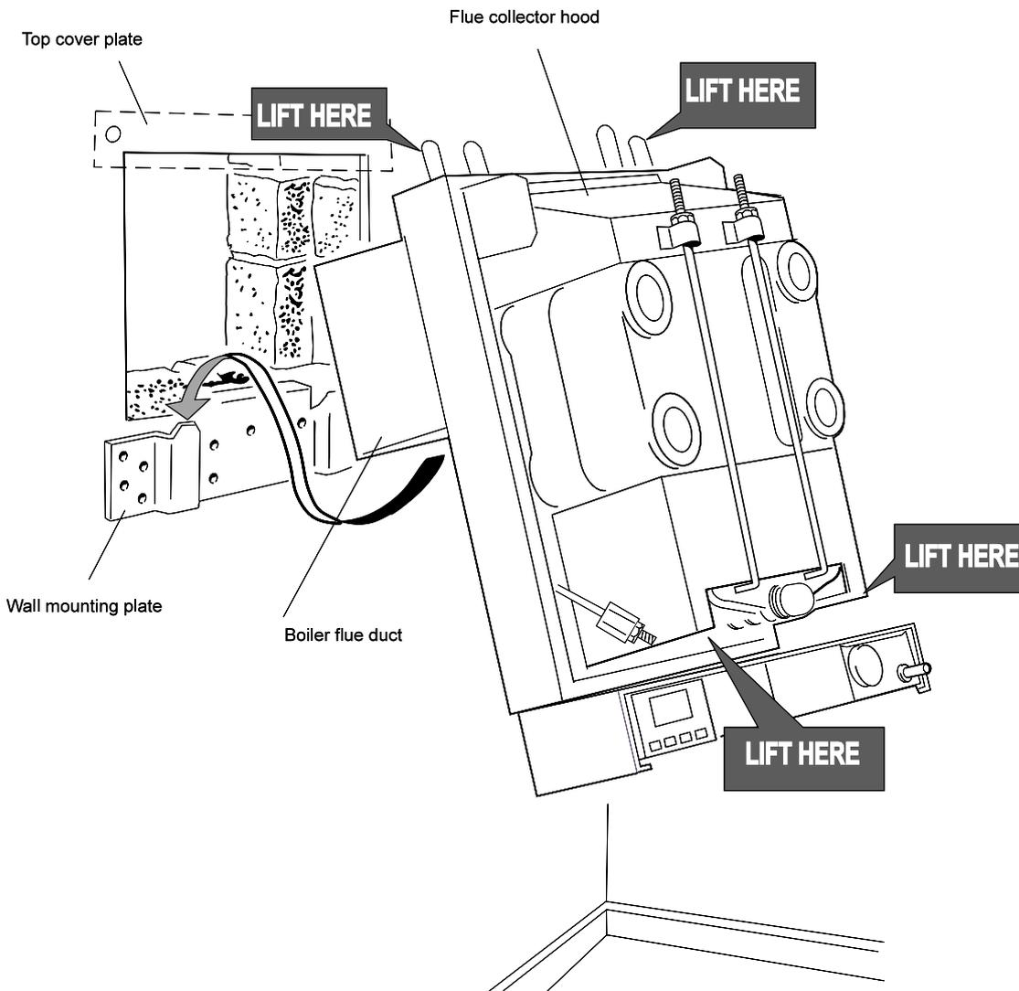
**Do NOT use the burner assembly for lifting**
