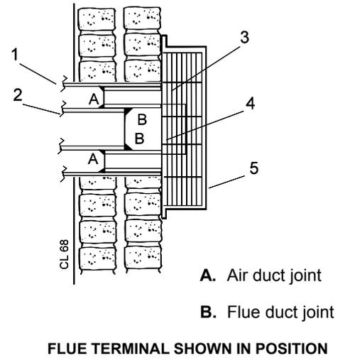
**Note.** For duct lengths greater than 400 mm (16") refer to Frame 14
