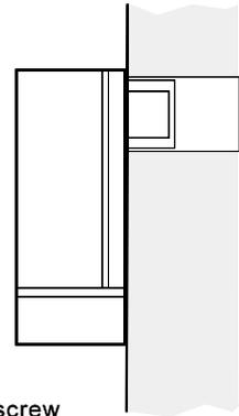
The flue duct should be horizontal
