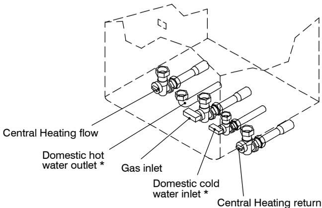
Connect to the tail pipes by proprietary fittings.
