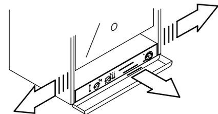
When completely pulled out, the panel can rotate 45° downwards to facilitate the operations on the internal parts.
