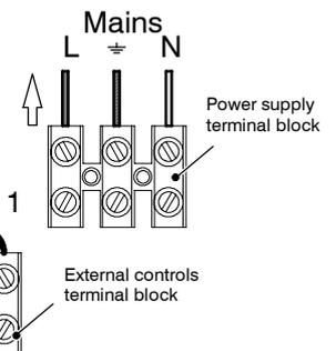
*Note: Ensure that the lengths of the current conductors are shorter than the earth conductor so that if the cable slips in its anchorage the current carrying conductors become taut before the earth conductor.*
