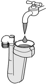
The condensate discharge system, pipework and fittings must be made of plastic. No other materials may be used. The discharge duct must have a gradient of 5 – 20 mm/m throughout its length. Condensate discharge via the gutter is not allowed given the risk of frost and the possible damage to materials
