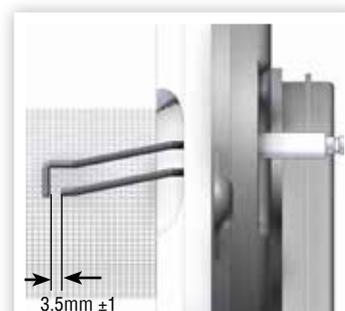
FIGURE 36. ELECTRODE GAP
