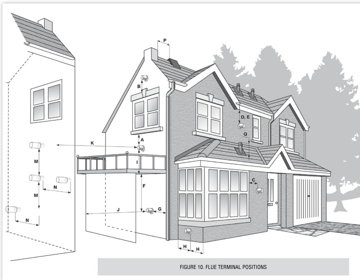
FIGURE 10. FLUE TERMINAL POSITIONS
