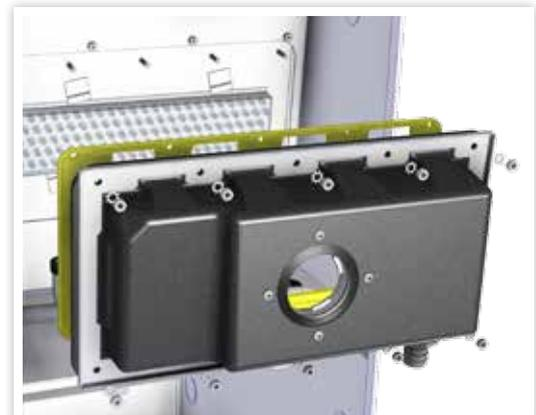
FIGURE 21. COMBUSTION AIR PASSAGE REMOVAL
