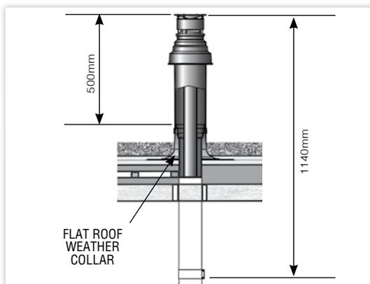
FIGURE 8. OPTIONAL ROOF OUTLETS
