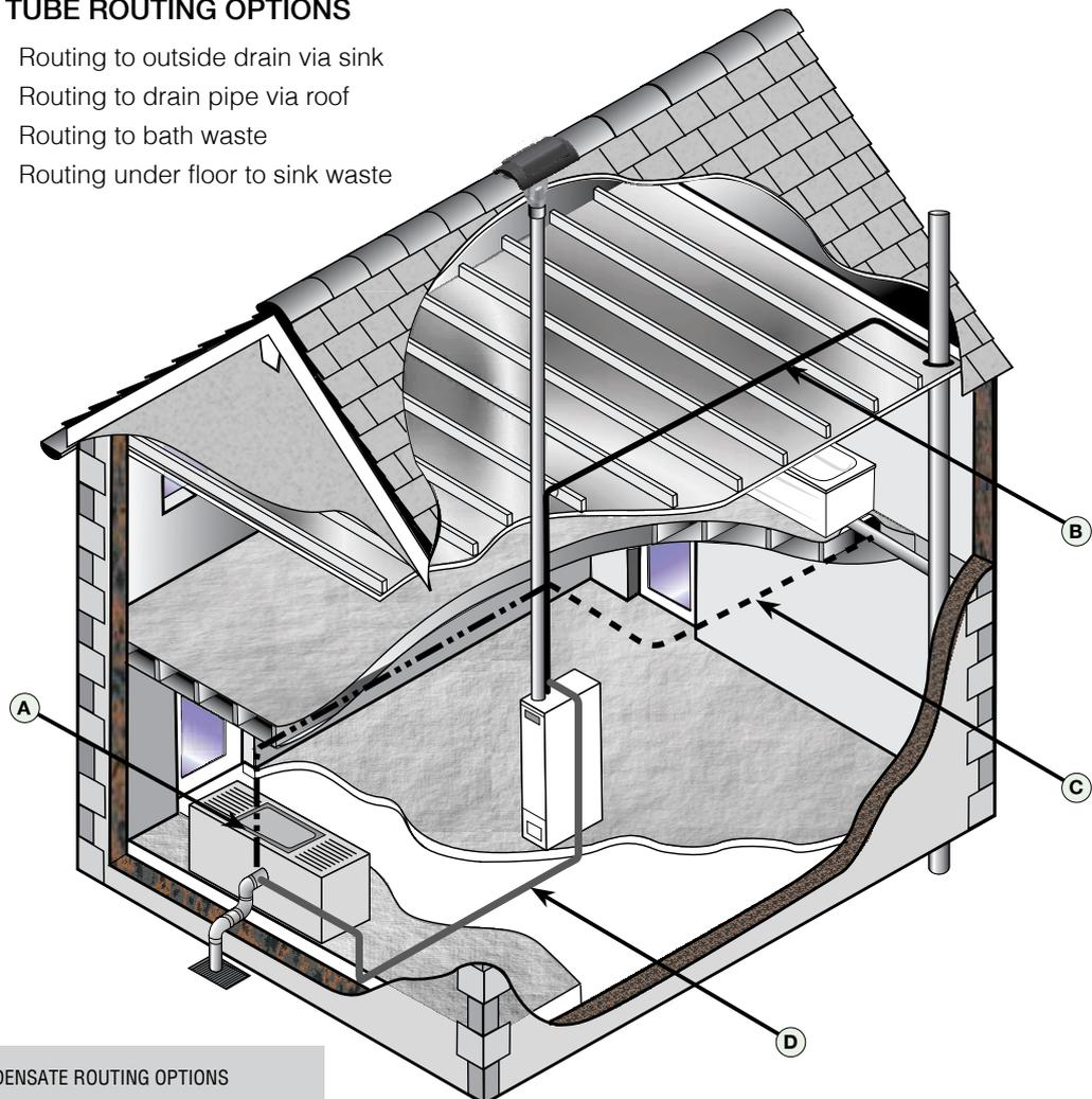
FIGURE 11. CONDENSATE ROUTING OPTIONS
