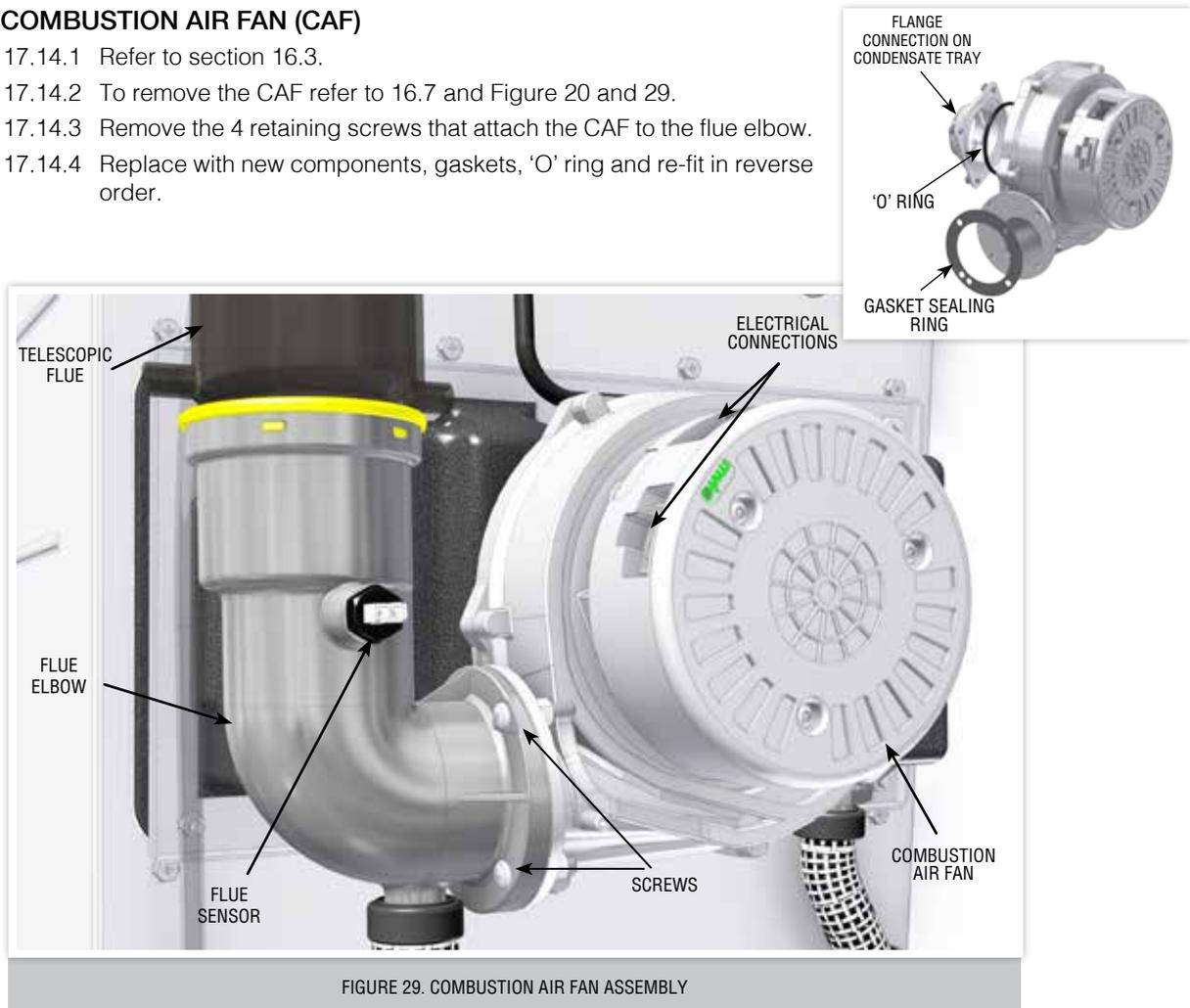
FIGURE 29. COMBUSTION AIR FAN ASSEMBLY
