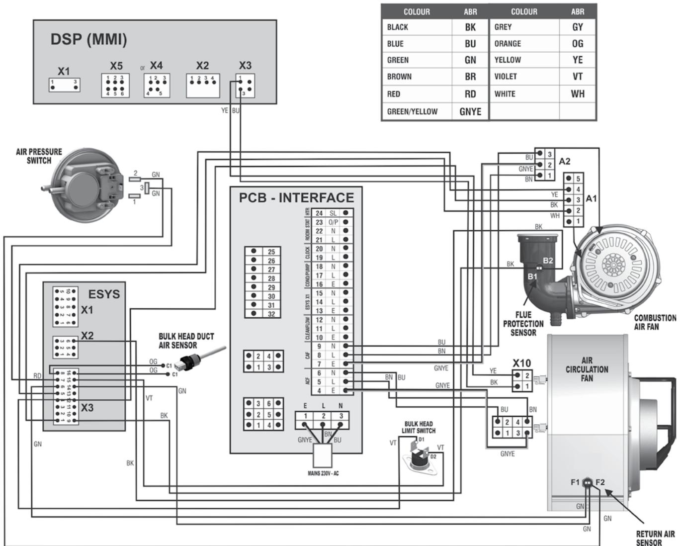
FIGURE 32. WIRING DIAGRAM No. 2 WIRING ROUTING TABLE
