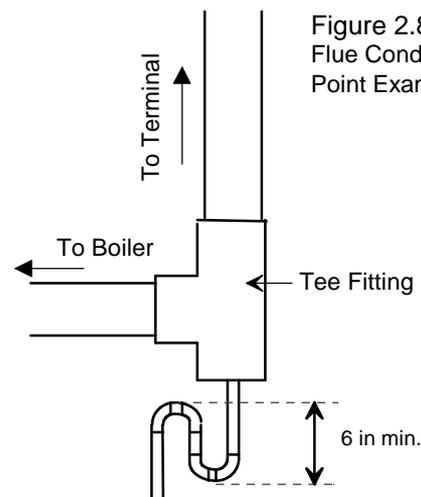
Figure 2.8.3 : Flue Condensate Drain Point Example
