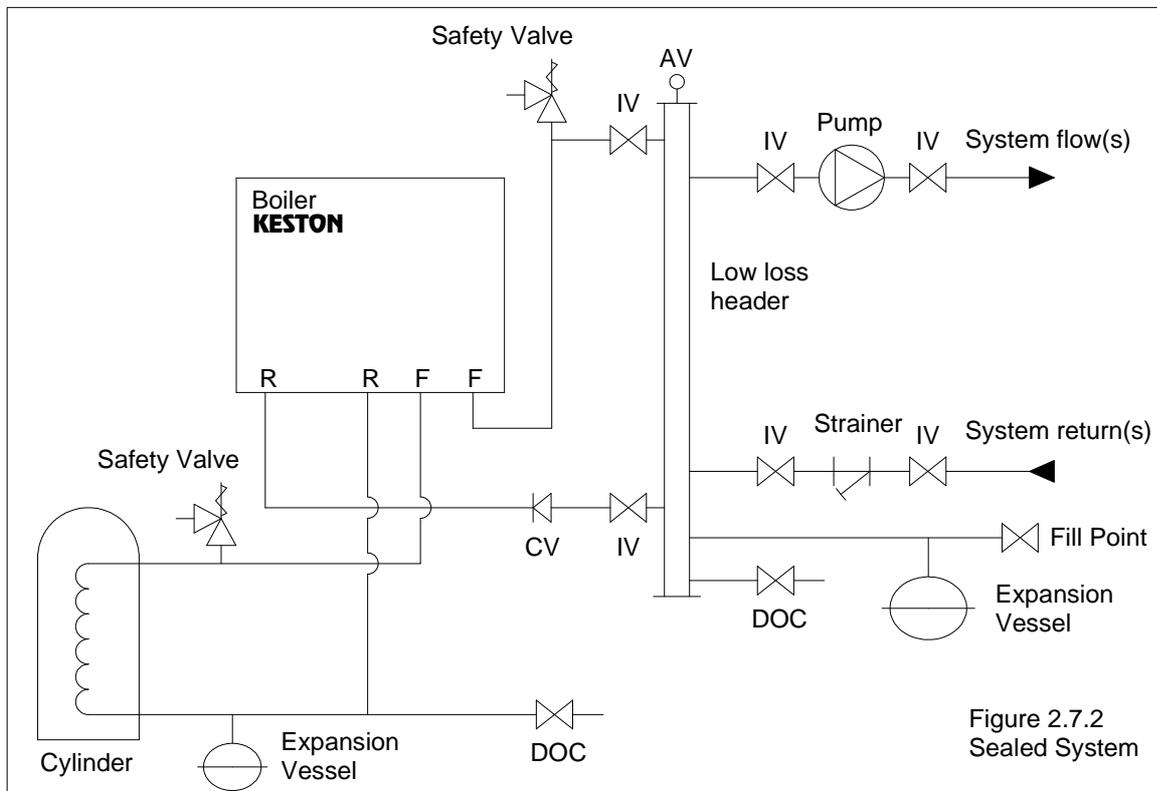
All components of the system including the heat exchanger of the indirect cylinder must be suitable for a working pressure of 3 bar and a temperature of 110 °C. Care should be taken in making all connections that the risk of leakage is minimised.
