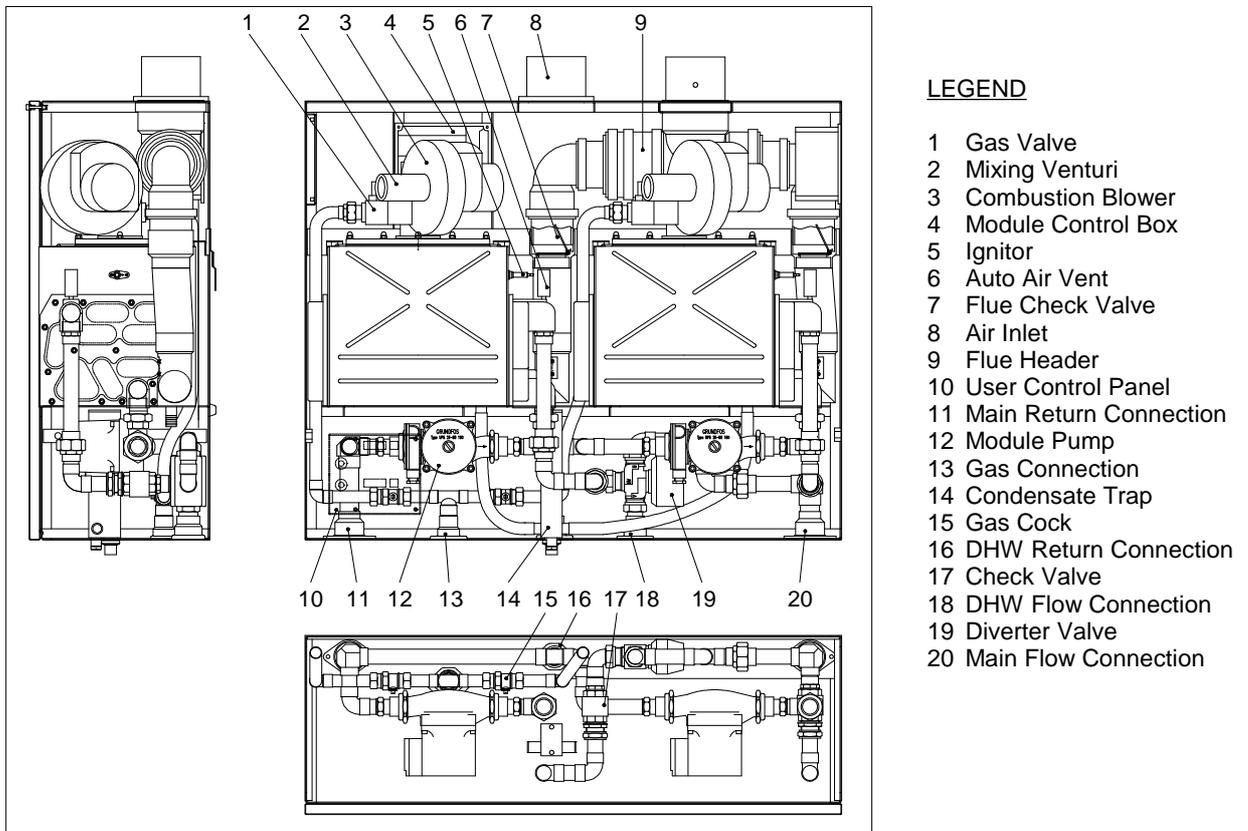
**Fig. 1.2 - Boiler Layout**
