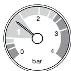
**Central Heating System Pressure** - The normal operating water pressure is shown when the needle is in the GREEN section of the gauge, between 1 and 2.5 bar. If the pressure exceeds 3 bar (needle in the RED section) the safety pressure valve will operate and a fault is indicated. Contact your Installer.
