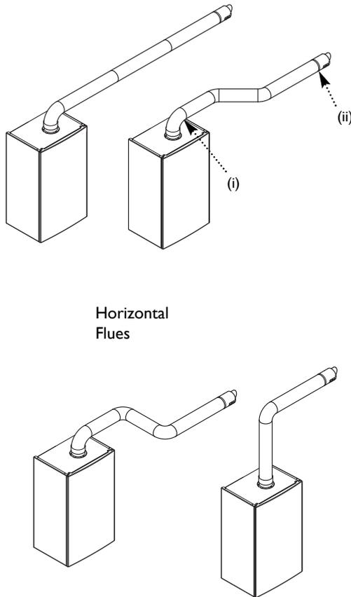
**NOTE:** Horizontal flue pipes should always be installed with at least a 1.5° fall from the terminal to allow condensate to run back to the boiler.
