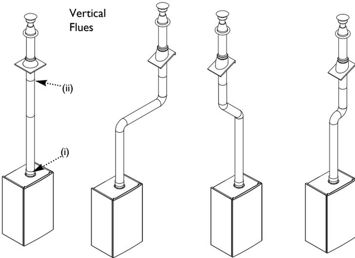
**IMPORTANT:** All flue systems must be securely supported at least once every metre. Suitable pipe supports are available as accessories.
