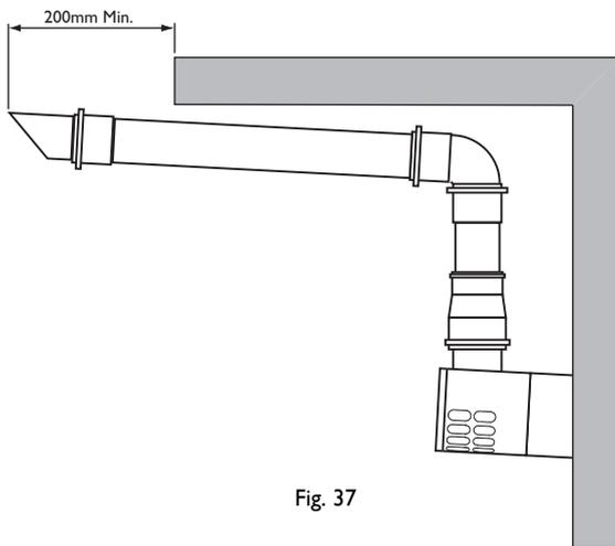
15. For aesthetic purposes it is permissible to route the 60Ø exhaust in an enclosed box, but the air inlet and plume outlet **MUST** remain in free air.
