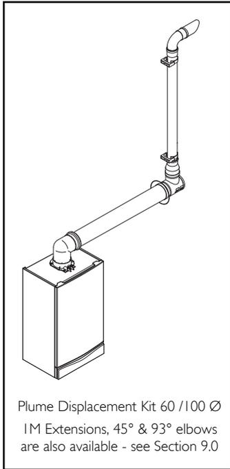
Plume Displacement Kit 60 / 100 Ø
