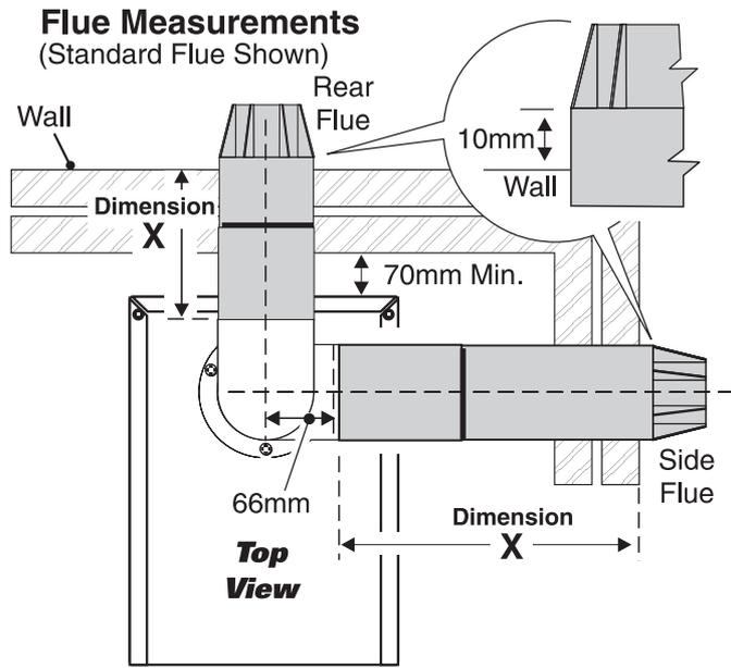
$$\text{Flue Length} = \text{Dimension X} + 20\text{mm}$$
