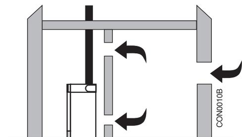
Open Flue Boiler Compartment
