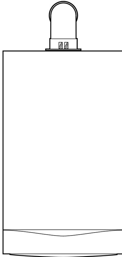
This is a Wall Mounted Powered Flue Condensing Combination Boiler Gas Fired Central Heating Unit.
