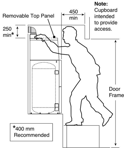
**Typical Bulkhead Installation with rearwards horizontal concentric flue**
