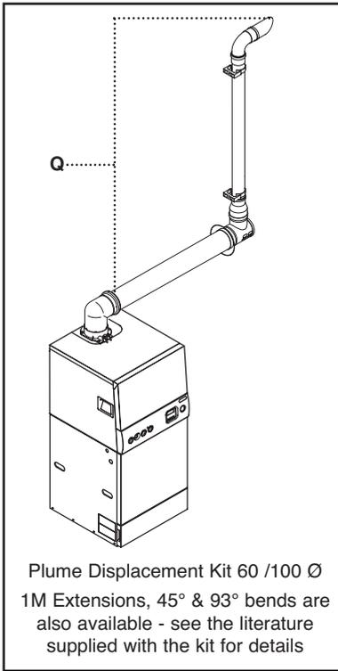
Plume Displacement Kit 60 /100 Ø
