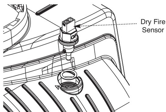
6. Disconnect the electrical connector and unscrew the sensor.
