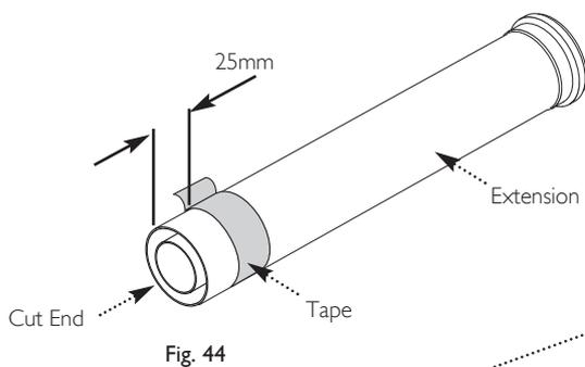
Apply Lubricant for ease of assembly. Ensure Extension is fully engaged into Boiler Adaptor
