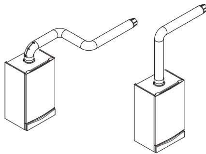
**NOTE:** Horizontal flue pipes should always be installed with a fall of at least 1.5° from the terminal to allow condensate to run back to the boiler.
