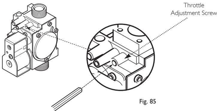
**NOTE:** To assist the boiler to light prior to final setting, use a suitable hexagon key to wind out the Throttle adjustment screw until it is flush with the valve body, then turn the screw 4 full turns clockwise (Fig. 85). If the boiler will not light, or the correct CO<sub>2</sub> cannot be achieved contact the 'heateam' technical helpline.
