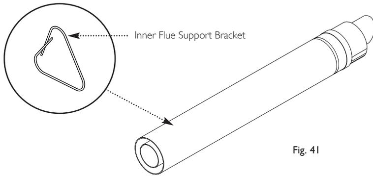
Apply Lubricant for ease of assembly. Ensure Flue is fully engaged into Flue Elbow
