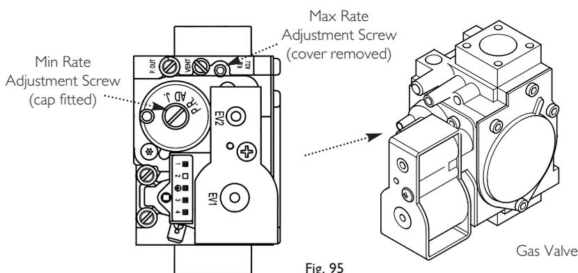
1. The combustion (CO<sub>2</sub>) may be checked after running the boiler for several minutes. To do this it is necessary to set the boiler to 'Calibration Mode'.
