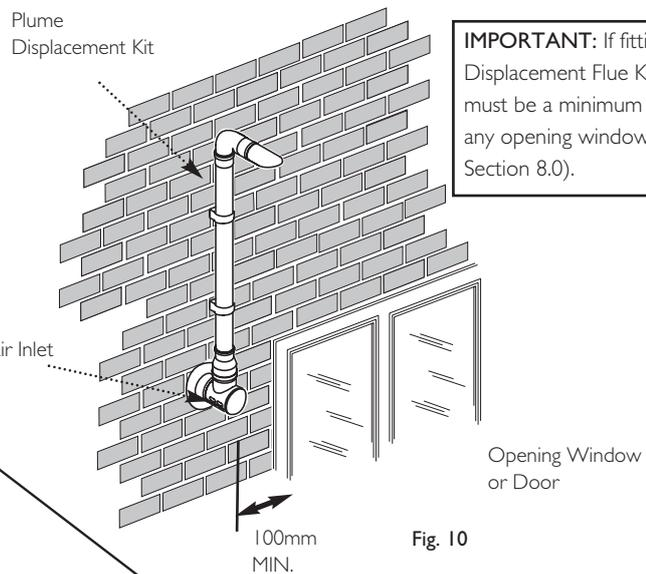
**IMPORTANT:** If fitting a Plume Displacement Flue Kit, the air inlet must be a minimum of 100mm from any opening windows or doors (see Section 8.0).
