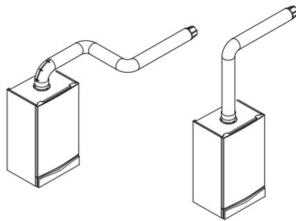
**NOTE:** Horizontal flue pipes should always be installed with a 1.5° to 3° fall from the terminal to allow condensate to run back to the boiler.
