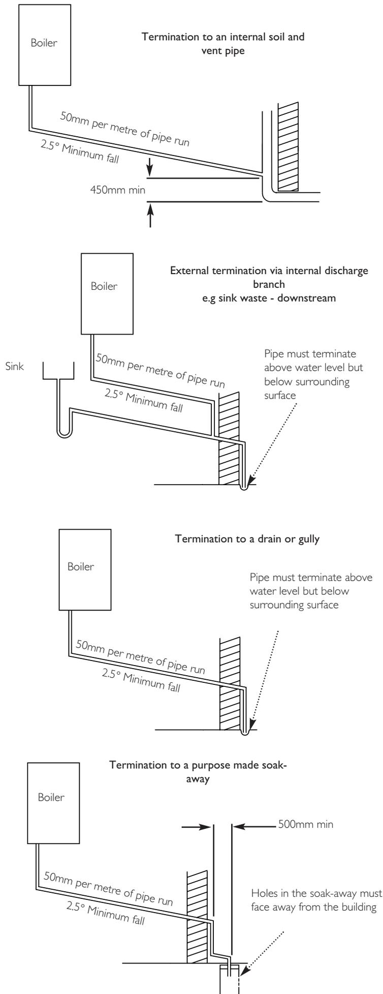
1. The condensate outlet will accept 21.5mm ( $\frac{3}{4}$ in) plastic overflow pipe which should generally discharge internally into the household drainage system. If this is not possible, discharge into an outside drain is acceptable.
