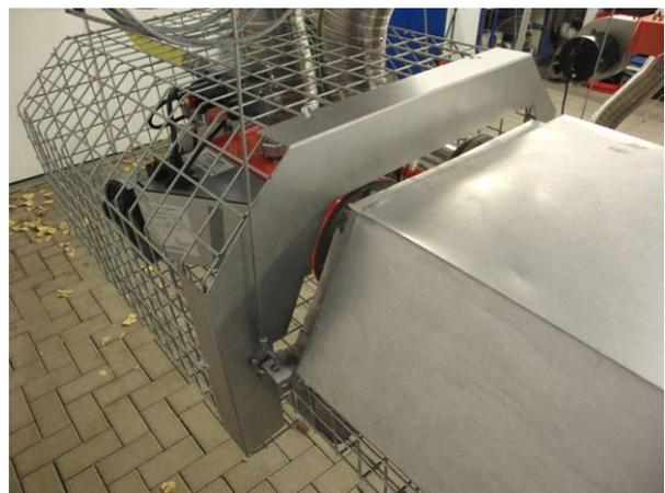
Fig. 55: Fixing front protection cover burner on protection grid burner top
