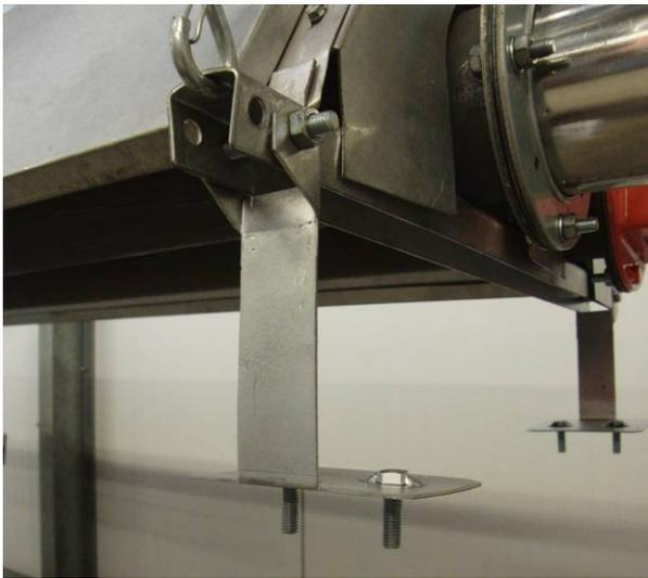
Fig. 51: Fixed angle bracket on suspension bracket
