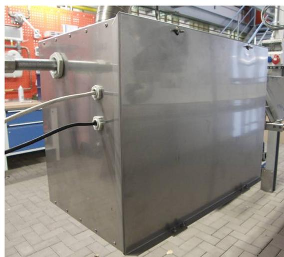
Fig. 64: Complete mounted and closed water protection cover
