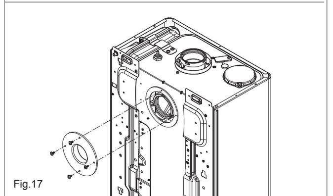
Using the screws and washers provided, secure the appliance onto the wall bracket and tighten with a suitable spanner. Seal the flue assembly to the wall using cement or a suitable alternative that will provide satisfactory weatherproofing. The exterior wall trim can now be fitted.
