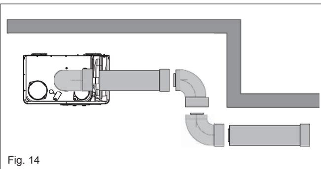
**4.5.1.2 FITTING THE REAR FLUE (fig. 15) (rear flue outlet only)**
