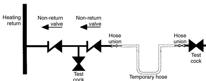
Fig. 6 Sealed primary water system - filling method
